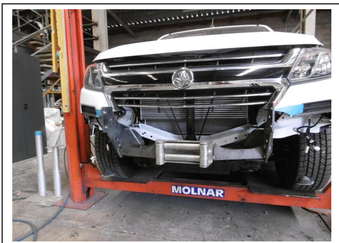
Figure 9: Winch frame fitted.
