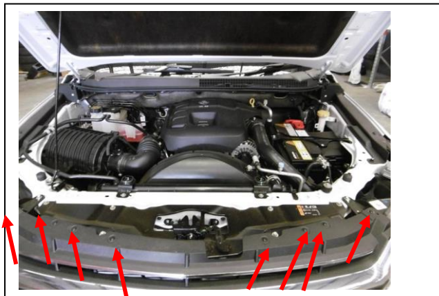
Figure 1: Remove grille screws.
