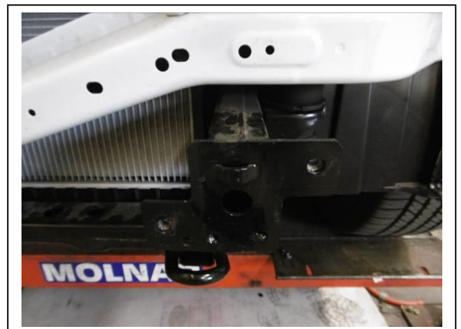
Figure 8: Flatten down tab.
